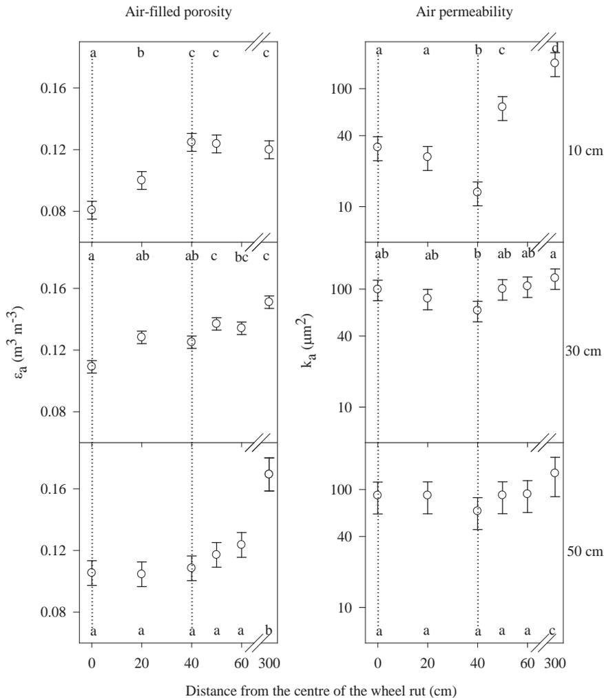
**Figure 1.** Air-filled porosity (left) and air permeability (right) measured at -100 hPa as a function of the horizontal distance from the center of the wheel rut at 10 cm (upper two figures), 30 cm (middle two figures) and 50 cm (lower two figures) depth. The dotted lines indicates the center and the periphery of the wheel rut.
