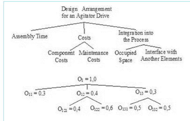
Fig. 5. Hierarchical objective tree for a stirrer drive design arrangement.
