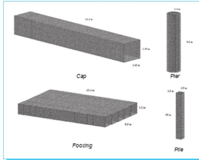
Fig. 3. Main bridge components.
