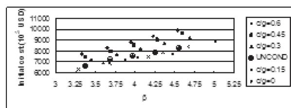
**Fig. 6.** Family of conditionals and unconditional initial cost curves for a bridge on the zone III, Mexico City.
