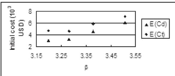
Fig. 11. Expected cost of failure and expected life-cycle cost for bridge Cuto.
