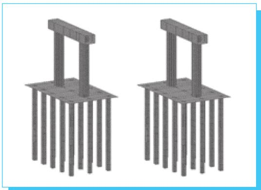
Fig. 2. Main supports of the bridge.
