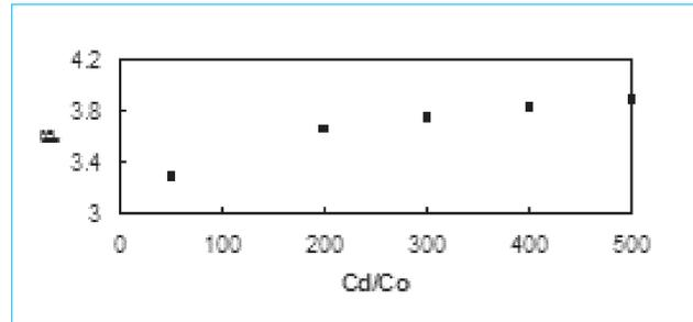
Fig. 1. Bridge acceptable reliability as a function of the ratio  $C_d/C_i$ .
