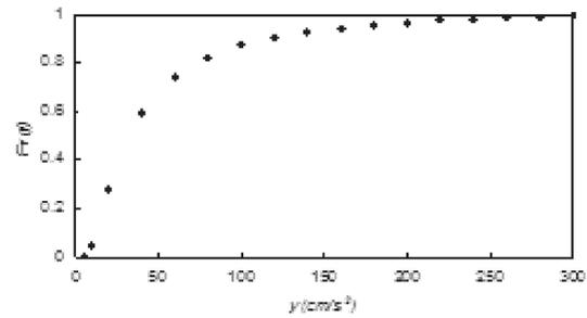
Fig. 9. Annual cumulative probability of seismic intensities for bridge Cuto.
