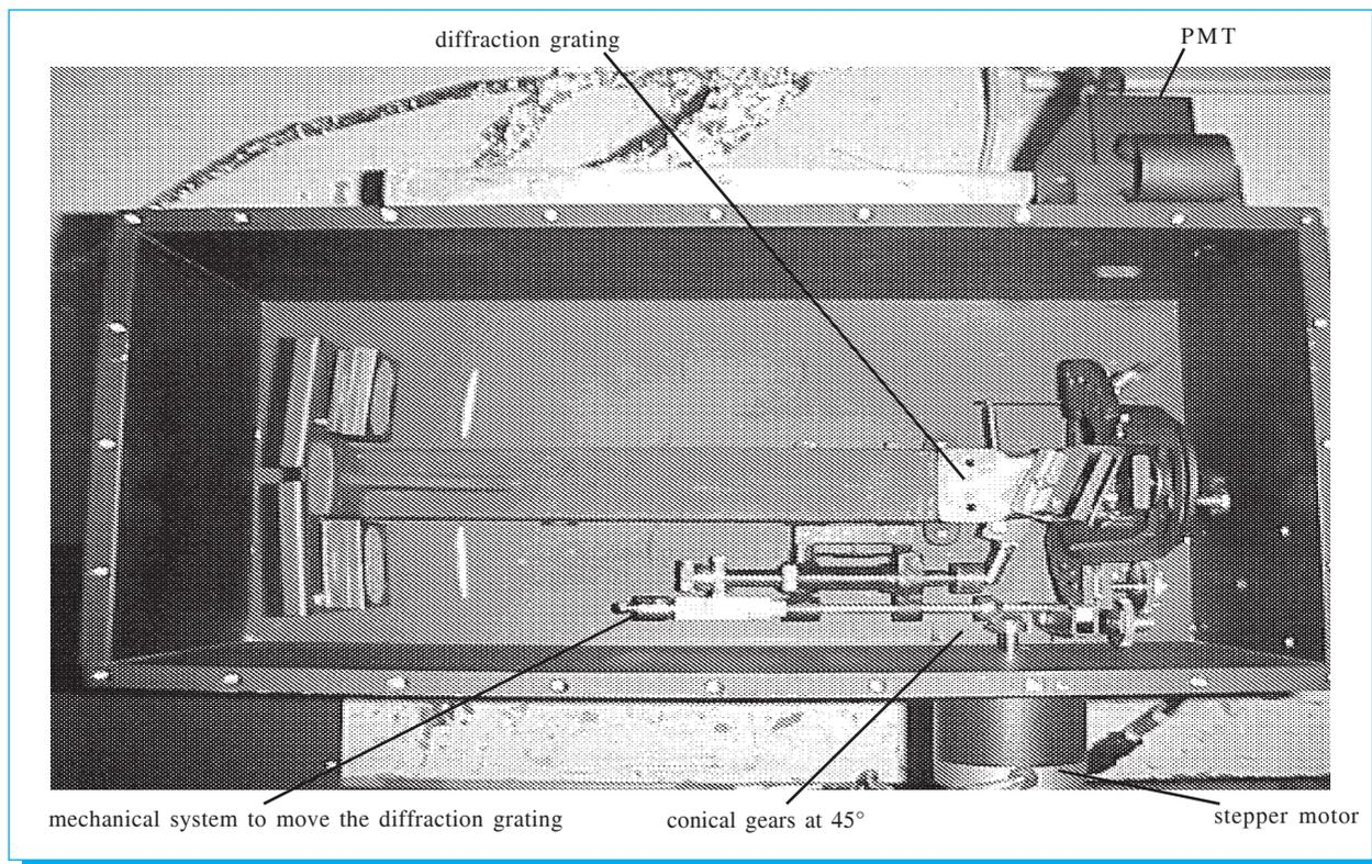
Fig. 3. Monochromator assembled in the chassis.
