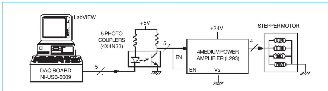
Fig. 4. Power circuits to move the stepper motor.
