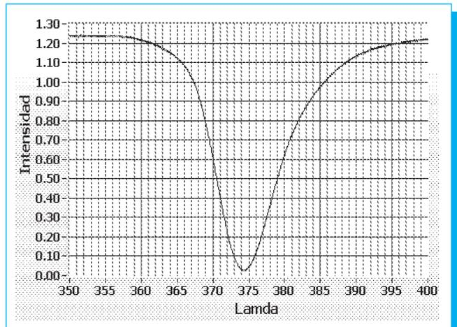
**Fig. 8.** Emission spectra of an ultraviolet led with a spectral width of almost 10 nm.
