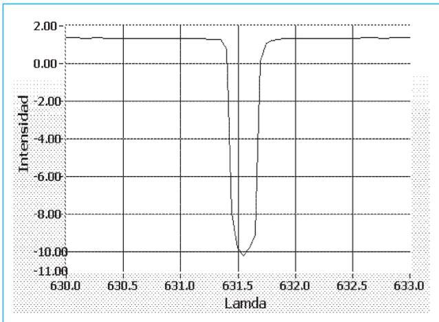
**Fig. 6.** Emission spectra of a helium-neon laser with high coherence and a spectral width of approximately 0.3 nm.
