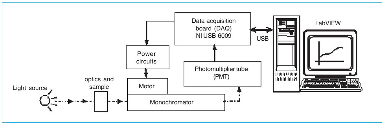
Fig. 1. Schematic diagram illustrating the developed spectrometer.
