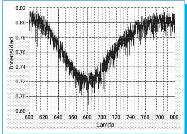
**Fig. 7.** Emission spectra of a standard red led without coherence and very dispersed.
