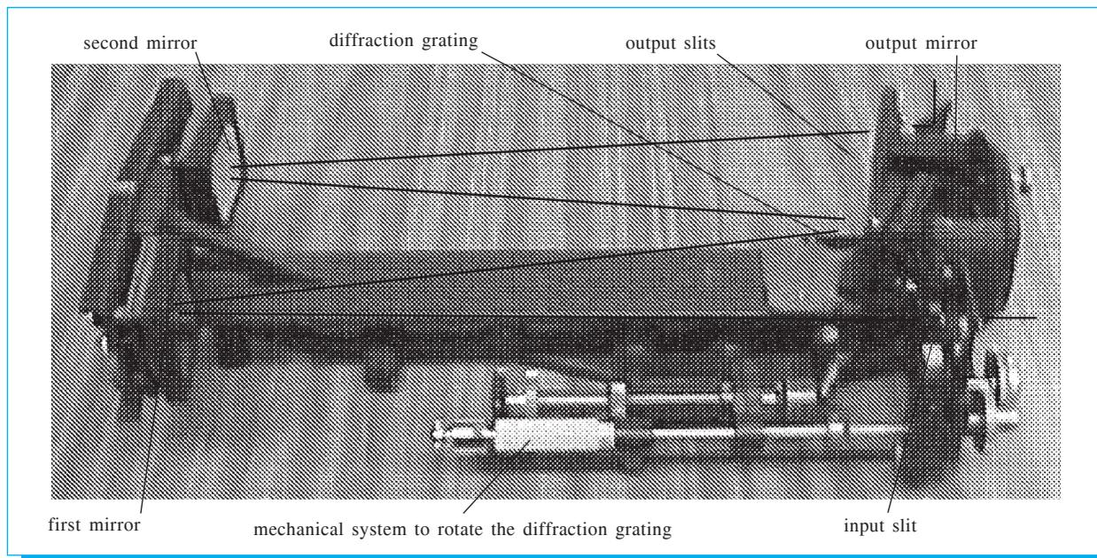
Fig. 2. Components of the monochromator used to develop the spectrometer.
