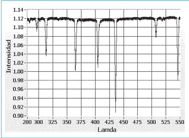
**Fig. 5.** Emission spectra of the mercury lamp with the spectrometer calibrated.
