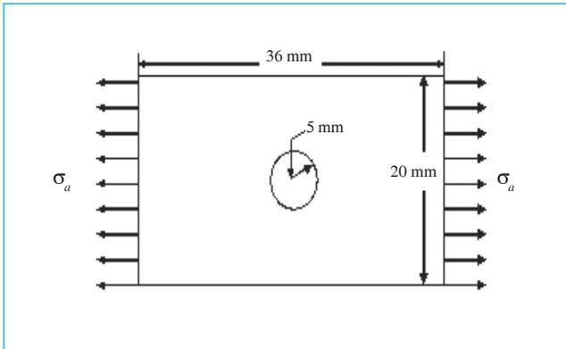
Fig. 3. Geometry and boundary conditions for a perforated plate.
