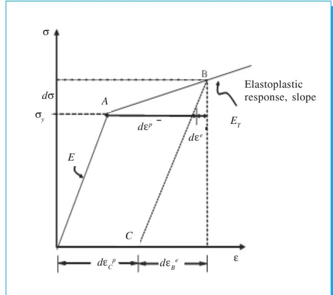
Fig. 1. Elasto-Plastic behaviour for a linear strain hardening.
