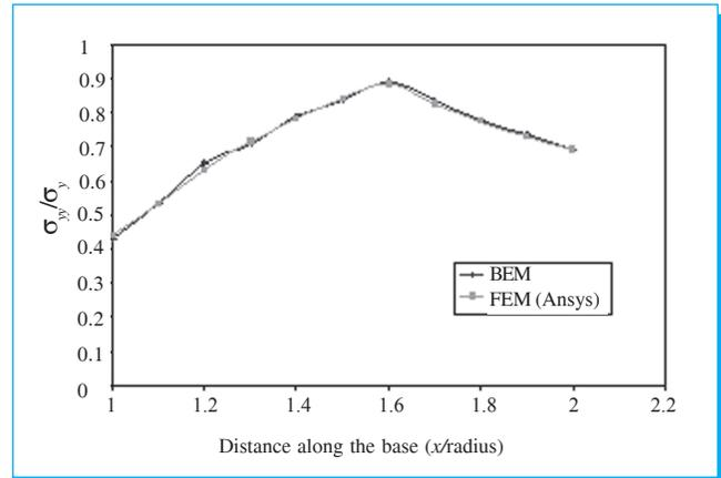
Fig. 8. Stress distribution of a thick cylinder on the base.
