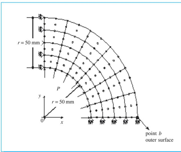
Fig. 4. Geometry, mesh and boundary conditions for a quarter cylinder under pressure.
