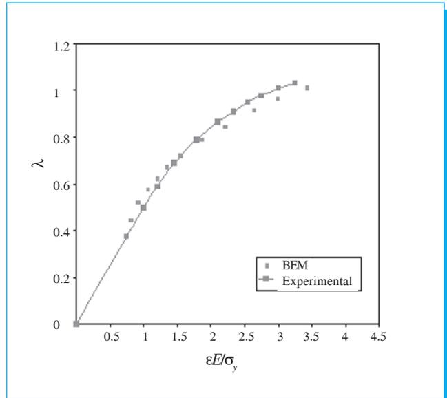
Fig. 5. Development of the deformation with the load factor.
