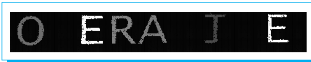
Fig. 4. Segmentation by connected component labeling of letters of a word from its image.
