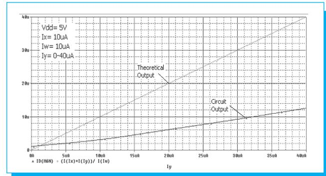
Fig.6. Simulation output of the multiplier/divider presented in [6] under the simulation conditions used in [3].
