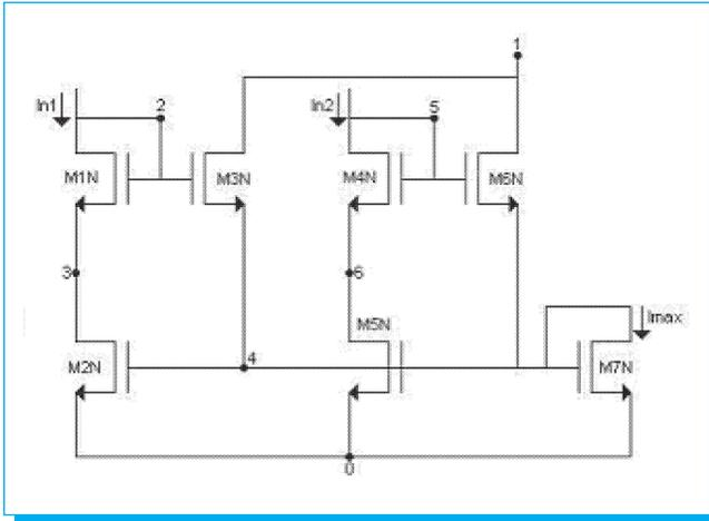
Fig. 22. Maximum detection circuit with two inputs.
