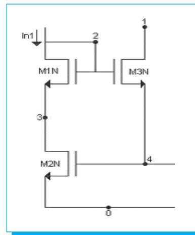
Fig. 21. Basic cell for the maximum detection circuit.
