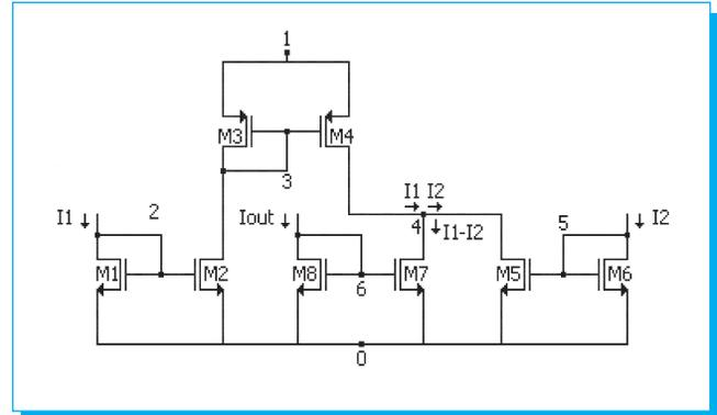
Fig. 1. Current subtract circuit.
