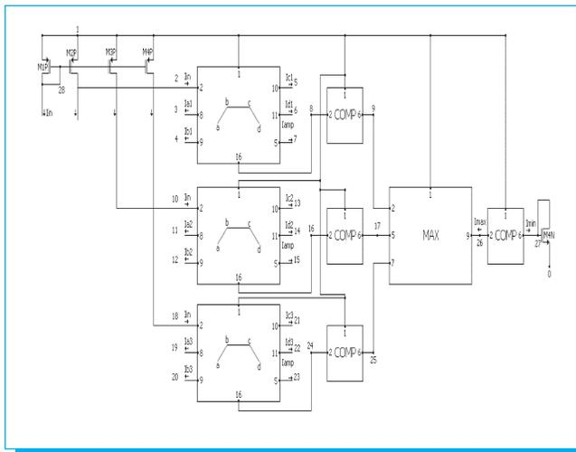
**Fig. 26.** Circuit used for the simulation of the minimum detection circuit.
