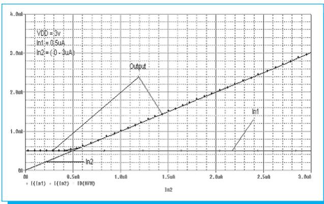
Fig. 23. Simulation output of the two input maximum detection circuit.
