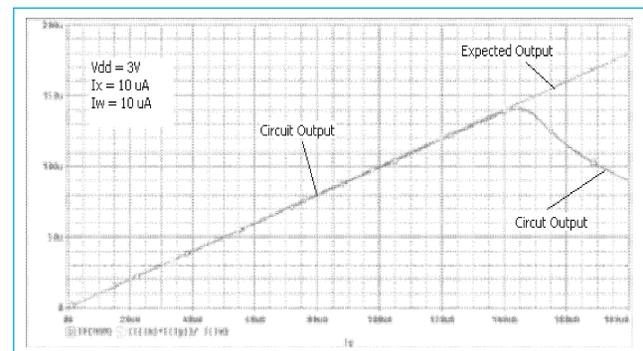
Fig. 8. Simulation output after proposed modifications.
