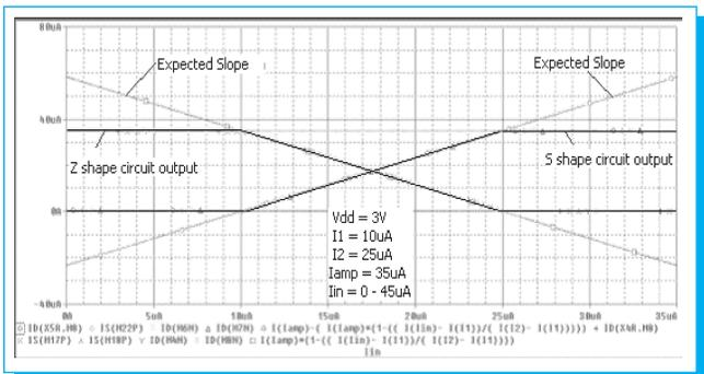
**Fig 13.** Simulation of the proposed S-Z shapes circuit.
