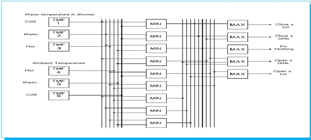
Fig. 30. Decision making system block diagram.
