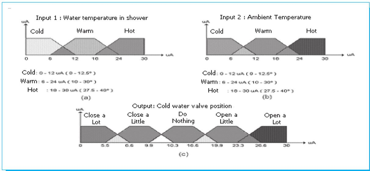
**Fig 29.** Membership functions for (a) Temperature in Shower (b) Ambient Temperature and (c) Output.
