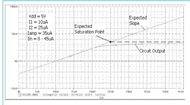
Fig. 11. Output error of the *S-Z* shapes circuit.
