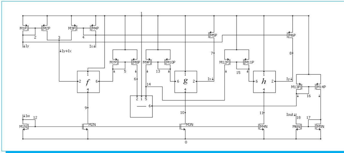
Fig. 7. Proposed quadratic-translinear multiplier/divider.
