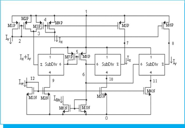
Fig. 5. Quadratic-translinear multiplier/divider.
