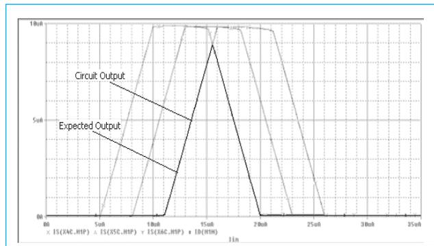
**Fig. 28** Simulation output for the minimum detection circuit
