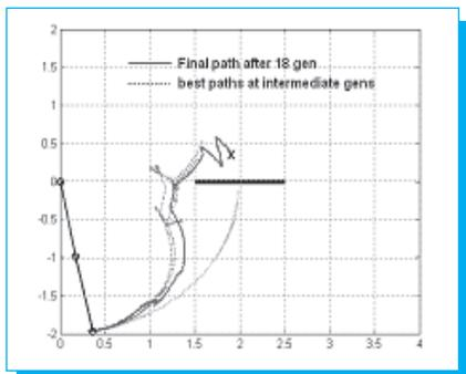
Fig. 14. Robot manipulator and paths obtained at different generations case II.
