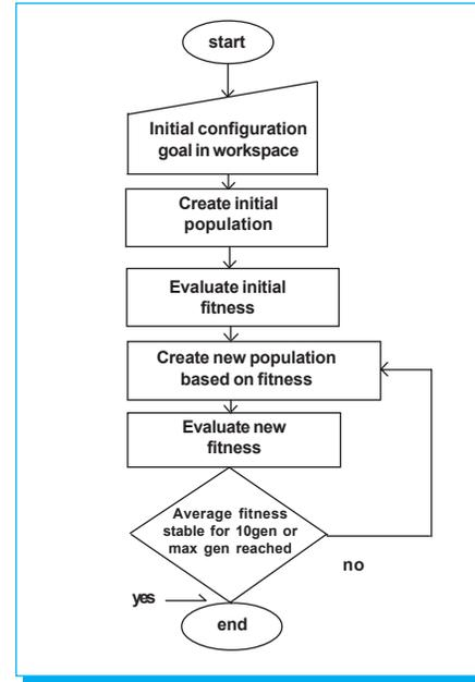
Fig. 11. GA based global path planning algorithm.
