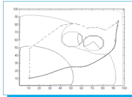
**Fig. 8.** Path comparison (dashed) conventional path planner (solid) GA path planner.
