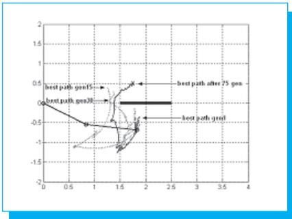
Fig. 13. Robot manipulator and paths obtained at different generation case I.
