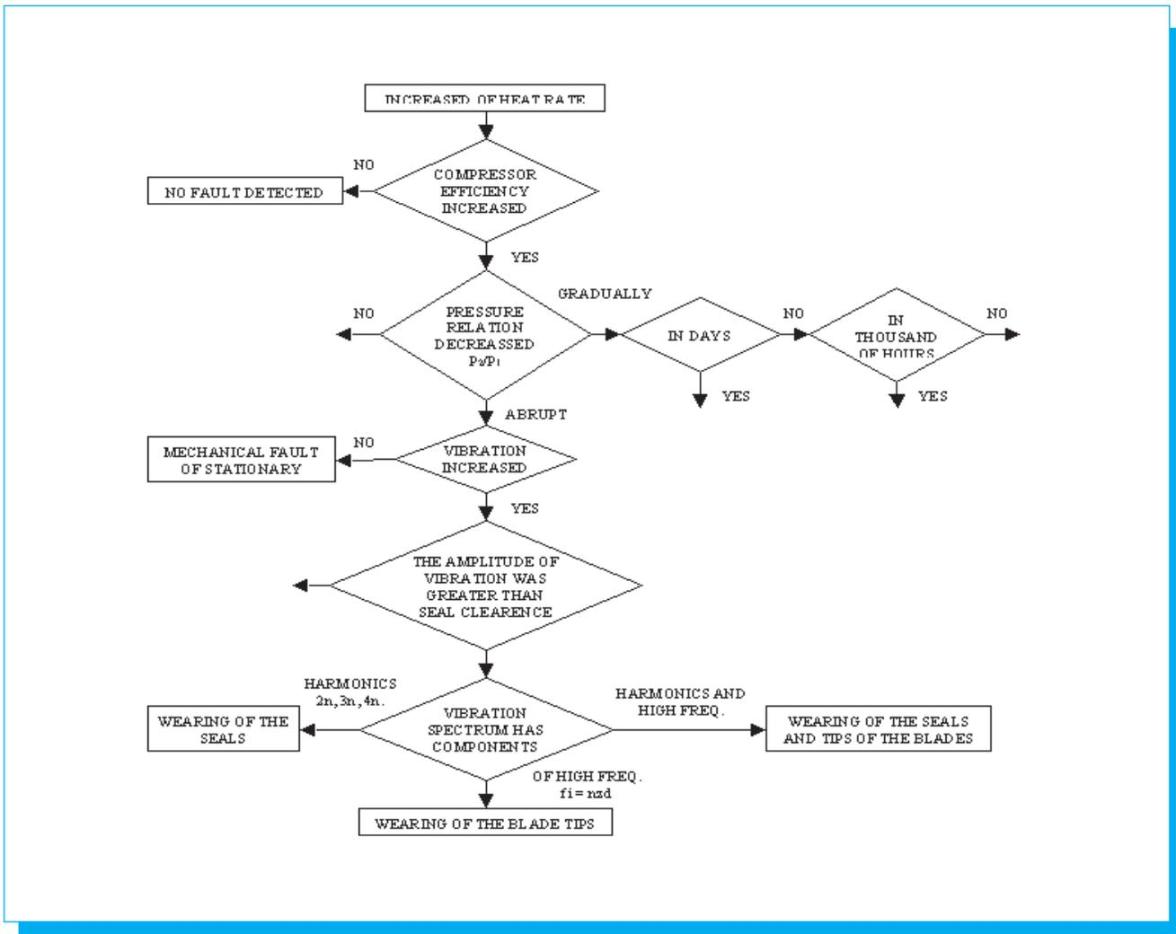
Fig. 5. Diagram of the turbocompressor faults identifications algorithm.
