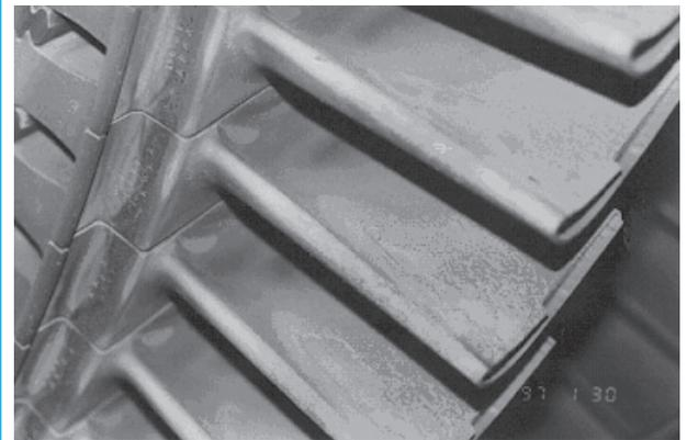
Fig. 1. Increase in roughness of the blading surface.
