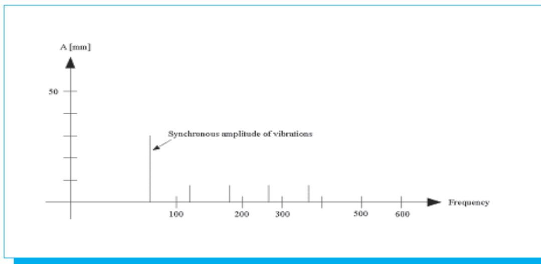
**Fig. 2.** The spectrum of the vibrations with pronounced harmonics.
