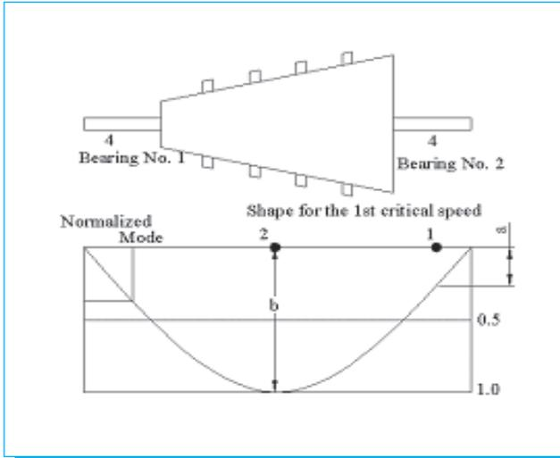
**Fig. 4.** Using critical speed program for determination of amplitude of vibrations at any point of the rotor. Measurement point 1", calculated point 2". Example: Vibrations measured at point A = 3 mils, Then the vibration at point 2" pointing the critical speed on A2 = An = b/a = 3(10/0.1) = 30 mils.
