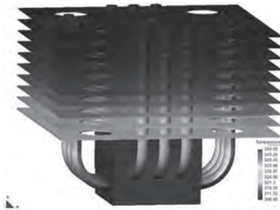
Figure 14. Resulting temperature distribution.
