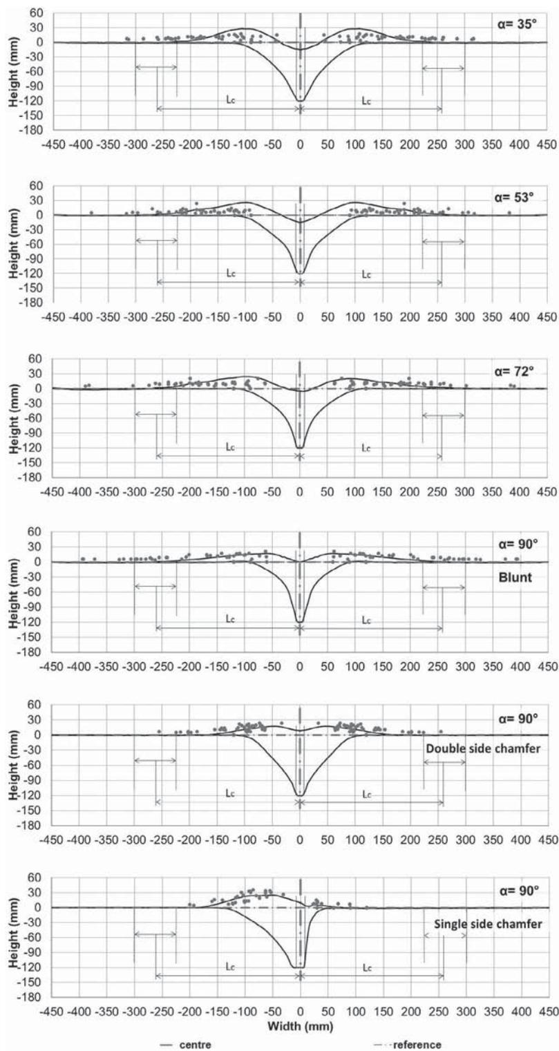
Figure 3. Cross section of soil profiles and tracer locations for various rake angles and different leading edge conditions.
