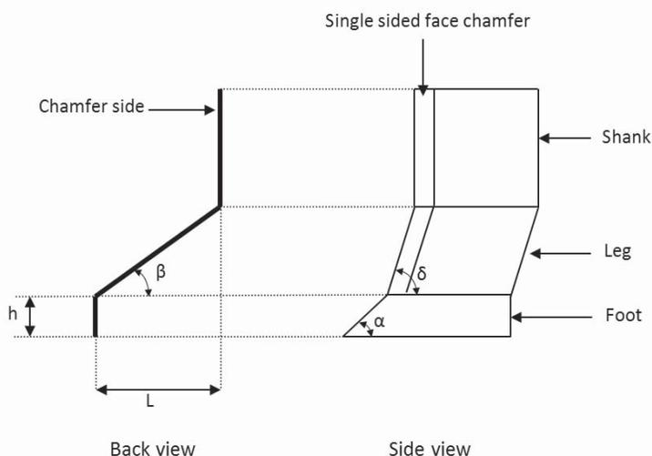
**Figure 2. Geometry of bent leg opener (L = shank lateral offset, h = foot height,  $\beta$  = side bend angle,  $\alpha$  = foot rake angle and  $\delta$  = leg forward angle).**
