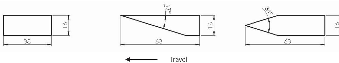
**Figure 1. Opener leading edge conditions evaluated on a 90° rake angle opener - blunt (left), single sided chamfer (middle) and double sided chamfer (right) - dimensions are in mm.**
