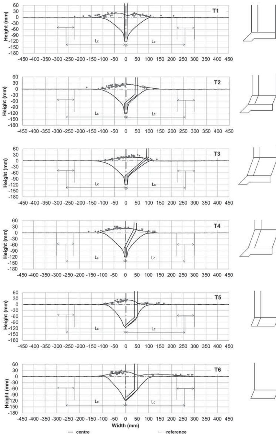
Figure 4. Cross section of soil profiles and surface tracer locations for various bent leg openers (corresponding opener side views are shown on the right hand side)
