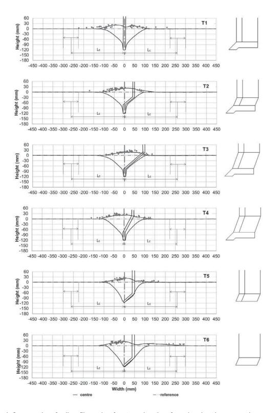
Figure 4. Cross section of soil profiles and surface tracer locations for various bent leg openers (corresponding opener side views are shown on the right hand side)
