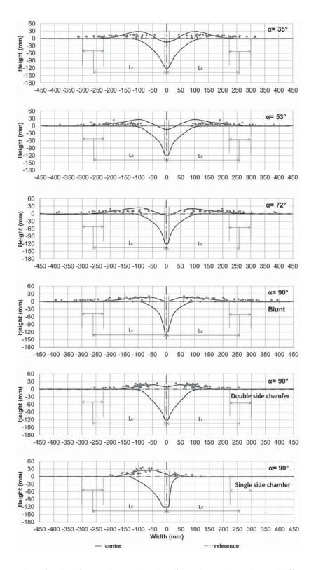
Figure 3. Cross section of soil profiles and tracer locations for various rake angles and different leading edge conditions.
