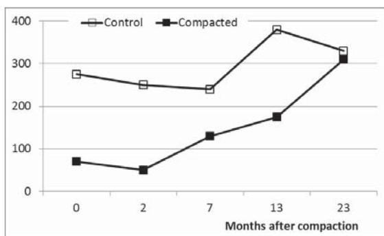
**Figure 3.** Number of macropores > 2 mm per m<sup>2</sup> at each sampling dates in under wheel tracks (compacted) and between wheel tracks (control) for two pore size classes.
