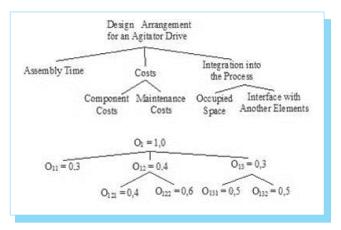
Fig. 5. Hierarchical objective tree for a stirrer drive design arrangement.
