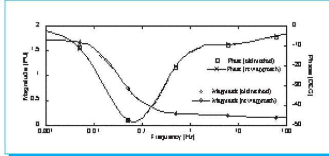
Fig. 15.  $d$ -axis operational reactance.
