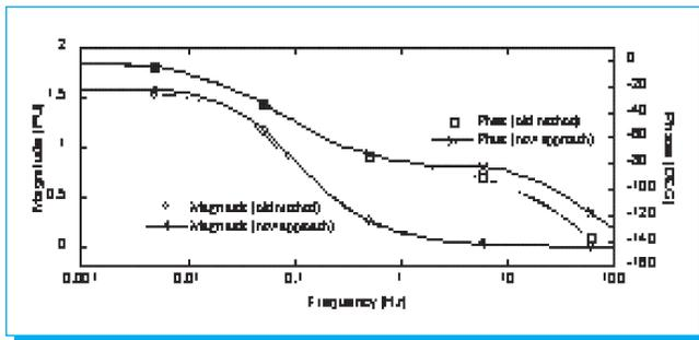
Fig. 17. Armature to field transfer reactance.
