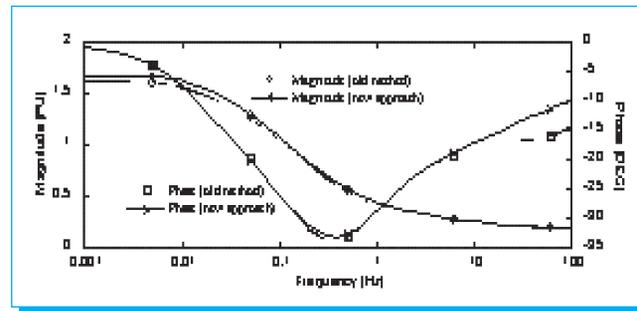
Fig. 18.  $q$ -axis operational reactance.
