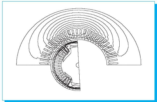
**Fig. 12.** Magnetic flux density distribution ( $\omega t = 0^\circ$ ) at 1 Hz.  $q$ -axis excited
