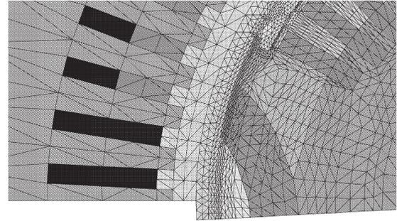
Fig. 4. Mesh zoom of the air gap region showing the different mesh densities of the rotor and stator domains.
