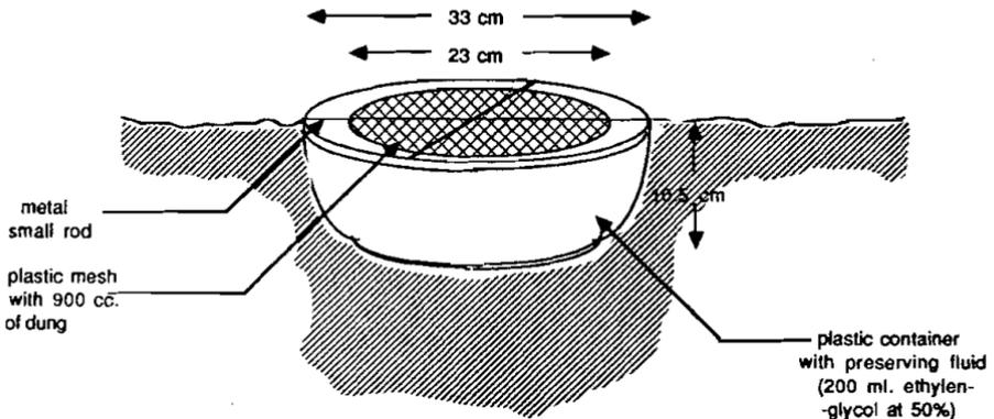
Fig.3. Details of the pit-fall used for following *Bubas bubalus* activity.
